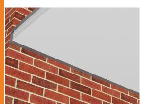
Seal joint upto 15mm between Corex and adjacent wall with FyreFLEX Sealant. Refer to page 15 for
